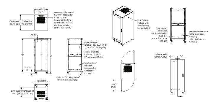
Note: side panels are required for door to lock/latch.
