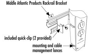
NOTE: Provided wood screws allow for mounting of mounting clip to wood surfaces
