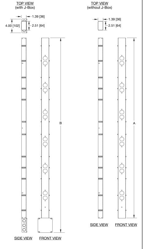
All dimensions in inches unless otherwise noted [bracketed dimensions in millimeters]
